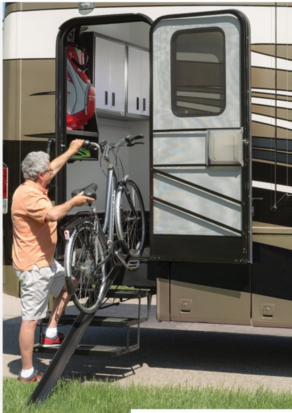
Side-Entry Door with Bike Ramp and Triple Steps
